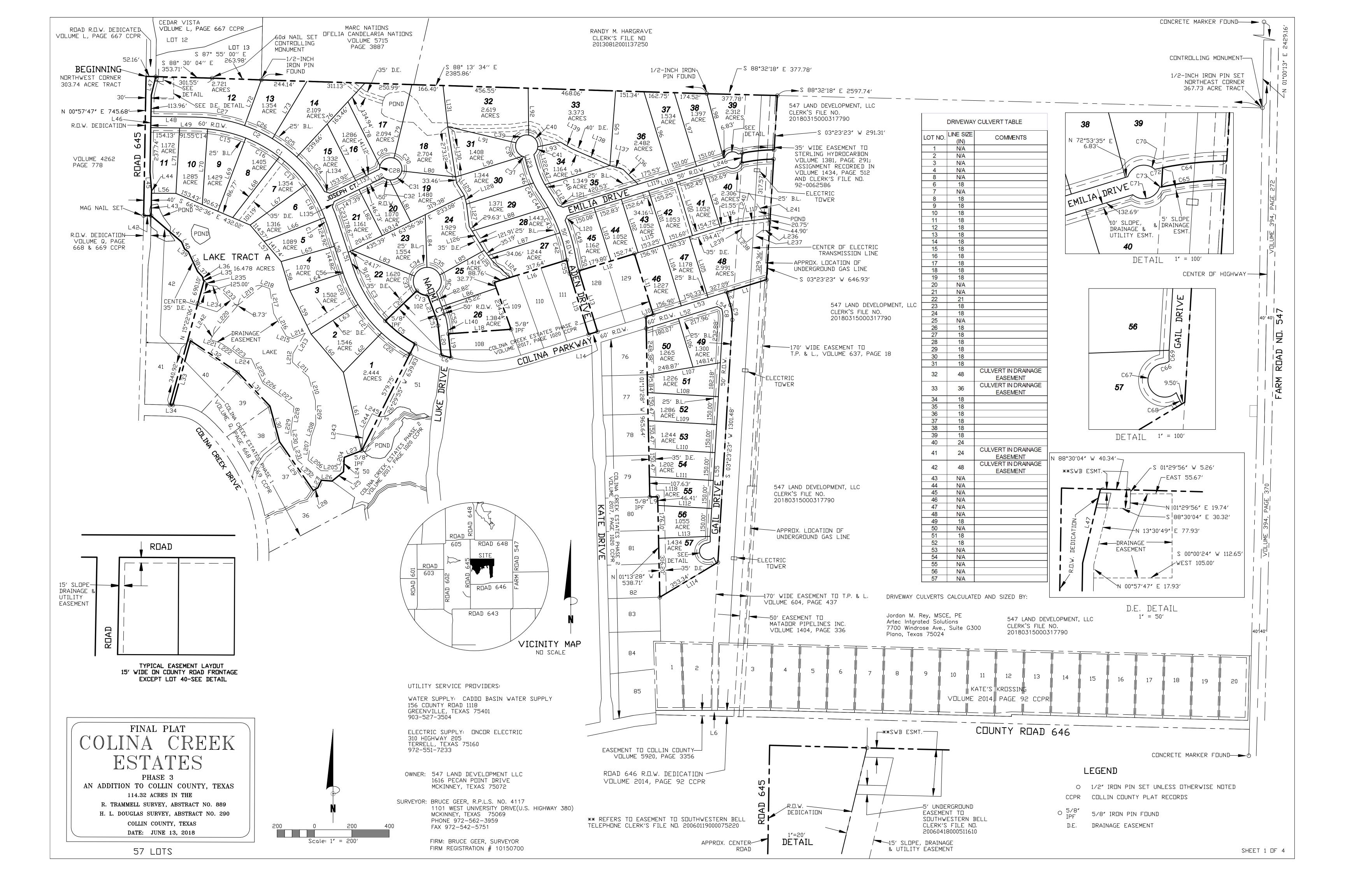
1. ANY OSSF THAT IS TO BE CONSTRUCTED WITHIN THE 100-YEAR FLOODPLAIN WILL REQUIRE SPECIAL PLANNING MATERIALS PRIOR TO PERMIT APPROVAL, 2. INDIVIDUAL SITE EVALUATIONS AND OSSF DESIGN PLANS PREPARED BY A
