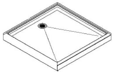
Cove base is required on three sides at the same height as the entry curb. Pan shall cap the entry curb down minimum 2".
