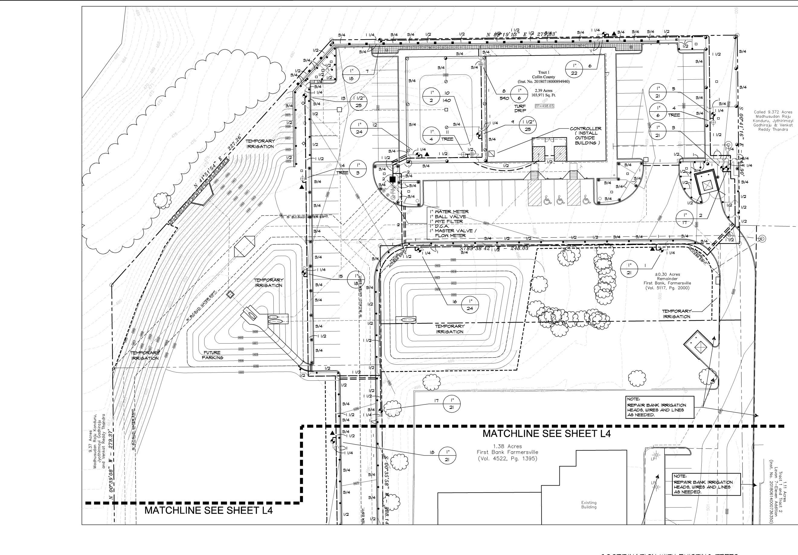
COORDINATION WITH EXISTING TREES NO MACHINE TRENCHING SHALL BE PERMITTED WITHIN THE ROOT ZONE OF EXISTING TREES. HAND-DIG ONLY, WITHIN THE ROOT ZONES OF EXISTING TREES. NO ROOTS OVER I" DIAMETER SHALL BE CUT. STAKE ALL PROPOSED TRENCH ROUTES NEAR EXISTING TREES FOR APPROVAL BY THE LANDSCAPE ARCHITECT BEFORE DIGGING BEGINS.
