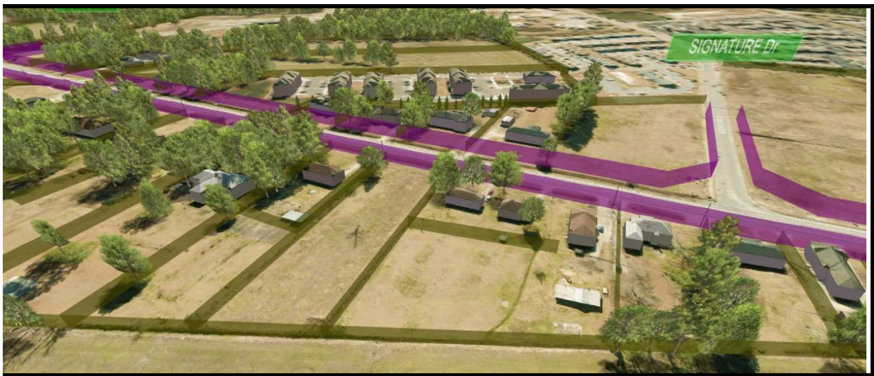
Figure 8 - Example of 3D Representation of ROW Lines and Property Boundaries
