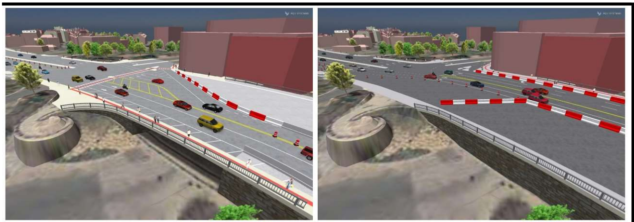
Figure 9 - Example of 3D Representation of Construction Staging and Maintenance-of-Traffic
