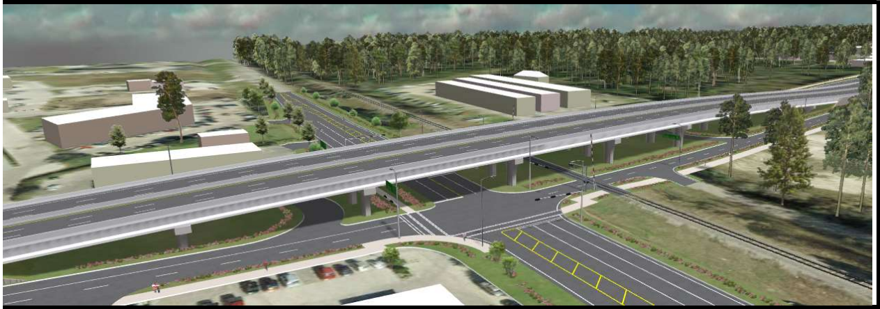
Figure 7 - Example of 3D Representation of Railroad Grade Separation
