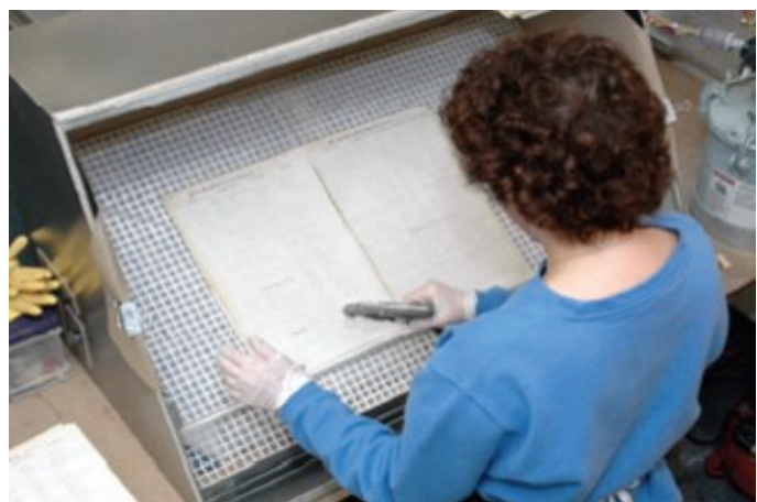
Non-aqueous deacidification with a fine mist on each side of the sheet.
