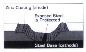
When Zinc is scratched the coating slowly sacrifices itself by galvanic action to protect the raw steel substrate.
